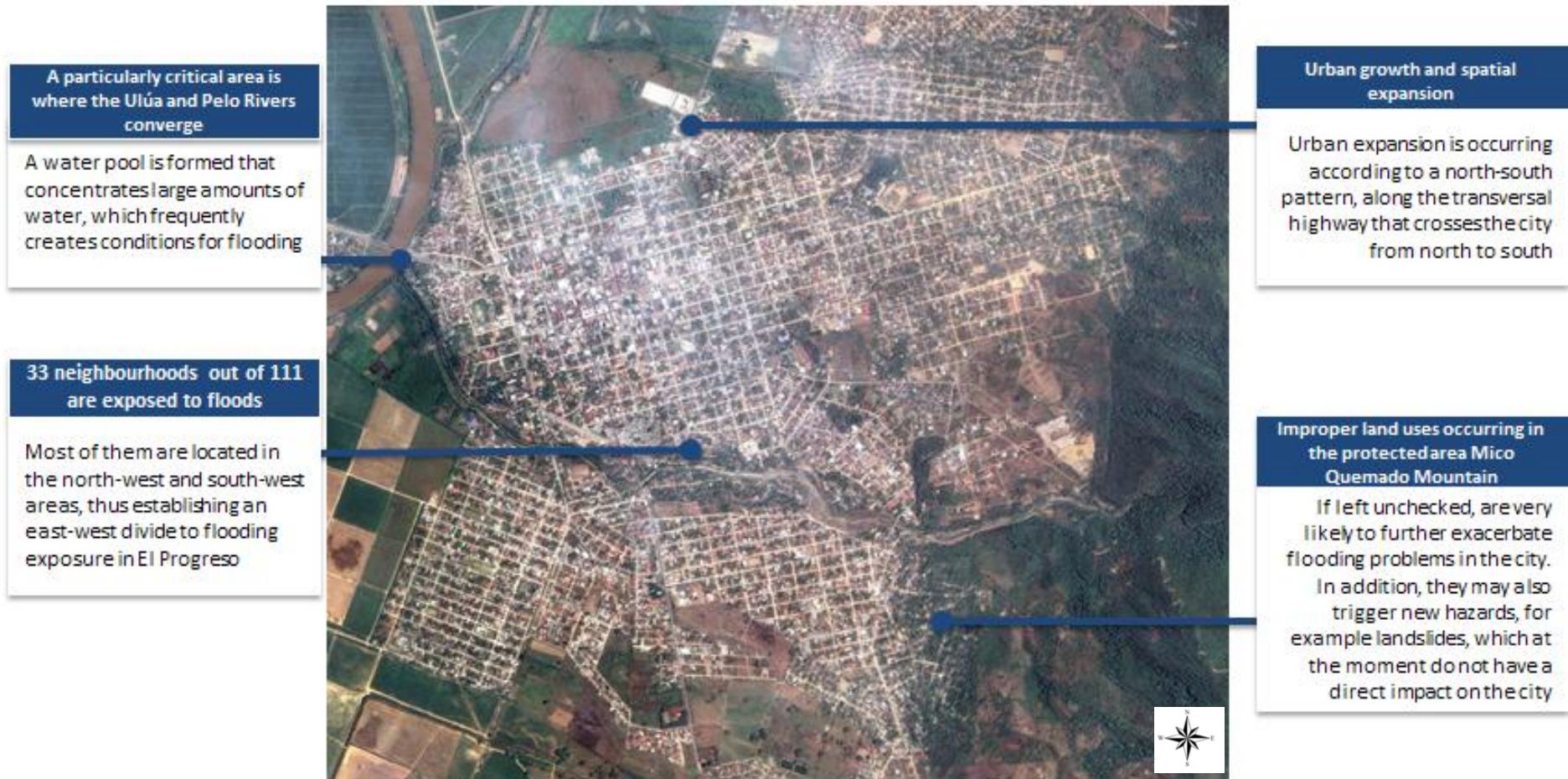
Figure 5.2 Predominant features of the built environment in El Progreso that impact upon flood and landslide hazard risks.
